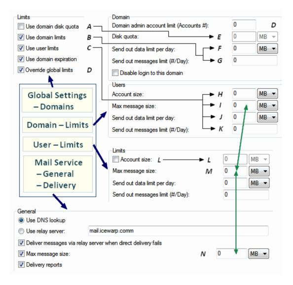
The diagram shows all the areas where limits are enabled and set. The straight arrows indicate a dependancy from one item to another, e.g. checking item of B (*Use domain limits*) will enable items of F and G (plus the *Disable login to this domain* box).
